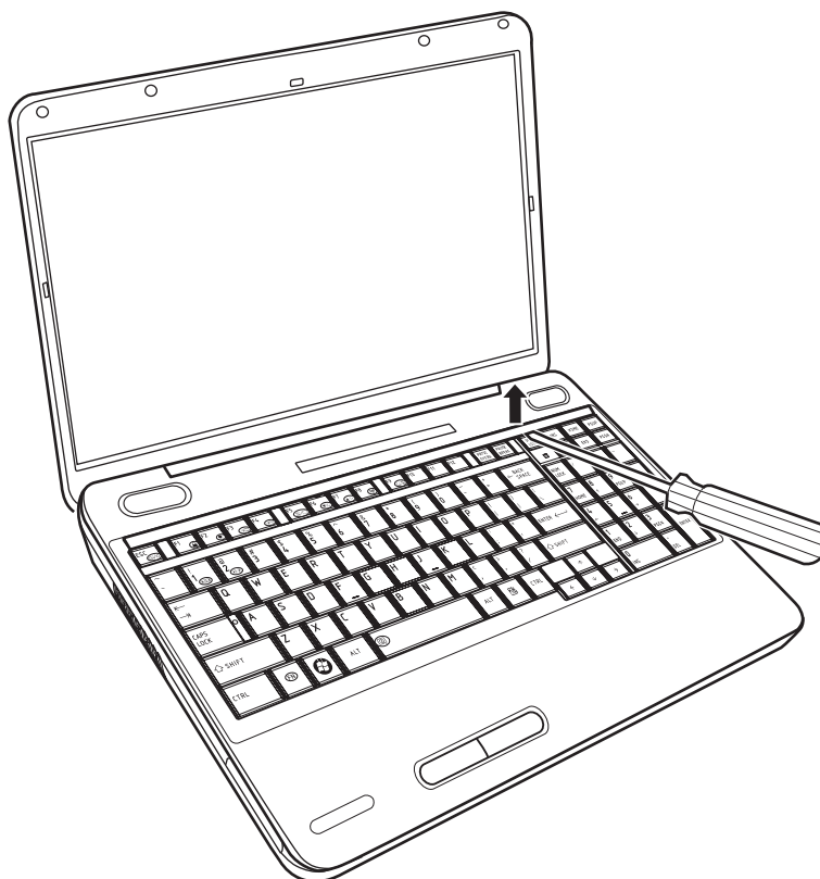
Figure 4.8 Removing the keyboard cover
